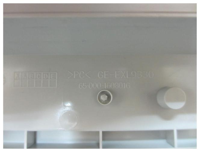
The main material of enclosure is PC material.
